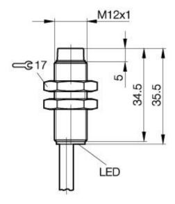
Inductive Sensors BES 516-356-E4-Y M12x1 x 37.5 normally-open Sn=4mm unshielded
